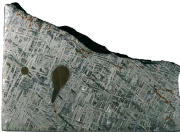
Figure 2. Polished and etched slice of the iron meteorite Carbo, which can be seen in the exhibition. Carbo was found in Sonora, Mexico in 1923. The 15 cm wide slice has a very clear, coherent Widmanstätten structure, which shows that it originally solidified as a single crystal. Just as the large Agpalilik slice Carbo contains brownish inclusions of the mineral troilite (FeS). The troilite solidified from sulphur-bearing melt inclusions that remained after the surrounding metal had solidified.
